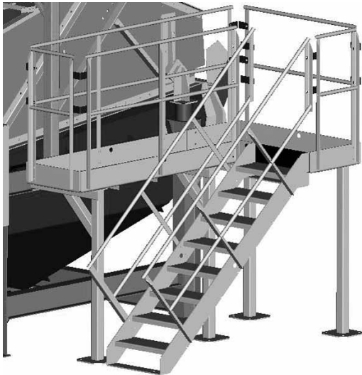
Walkway and steps for ease of maintenance
