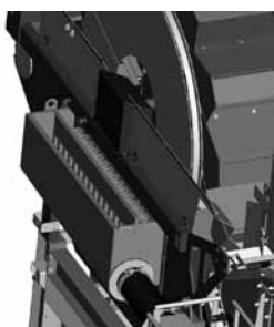
Weir discharge system
